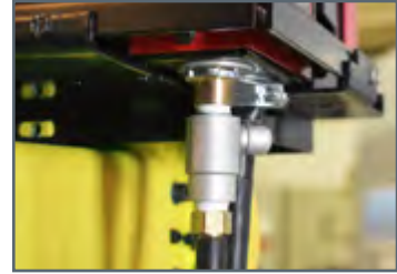
Installation at gas inlet on the wire feeder
