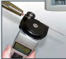
HHSS-12 obtaining measurement at the torch end
