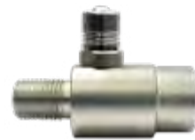
GFJ-ADJ-B 1/4"-18 Male NPT x 5/8"-18 Female NPT
