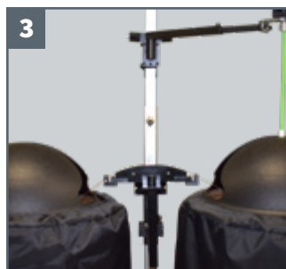
3 Position the wire on the pathway between the two drums.
