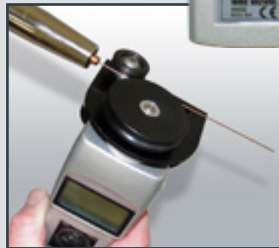
HHSS-12 obtaining measurement at the torch end
