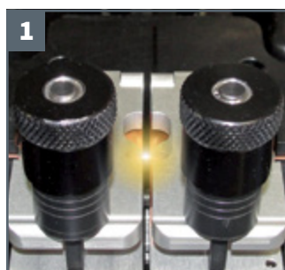
1 Join the end wire from drum 1 with the start wire from drum 2 using the Butt Welder.
