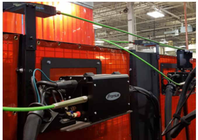
Wire Wizard® inlet guides, conduit and Wire Guide Modules were installed in this optimized wire delivery setup with wire feeders mounted in a fixed position outside the weld cell.
