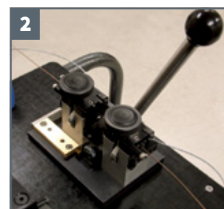
2 Remove the flash in the wire joint using the Wire Sizer (sold separately) or rotary tool with stone bit.
