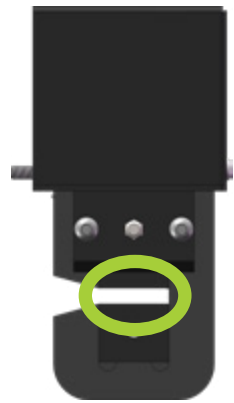
Figure 12 To extend Wire Cutter blade life, it is recommended to adjust the robot position inward or outward after each 10,000 cycles so blade is not cutting at the same location every time.
